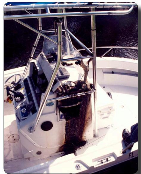
**When the owner of this boat added a light fixture, he neglected to add a fuse to the circuit. Fuses protect the wires from overheating and without one, chafe or a defective fixture can cause a fire (Claim # 9800883).**
