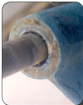
**Cutless bearings tend to be forgotten about, but after a few years of use, the inside lining wears and the bearing has to be replaced. There should be very little play when the shaft is moved side to side.**
